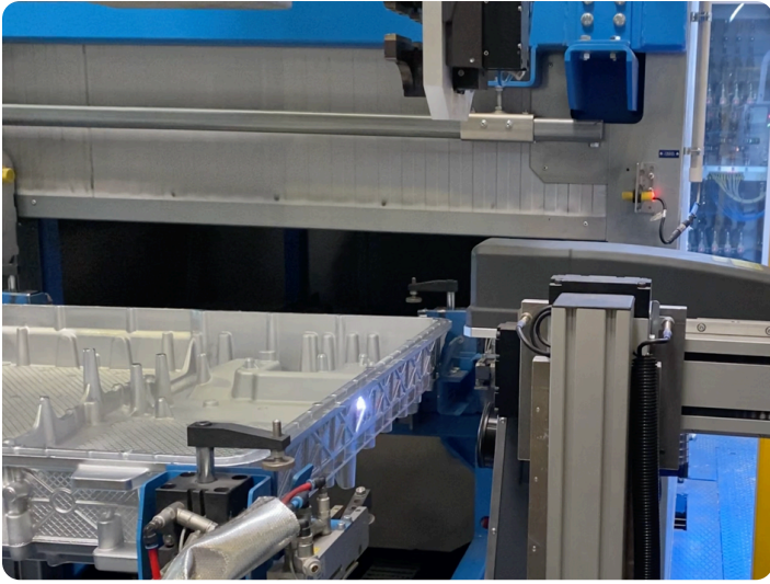
Marking CDOT code on cast aluminum
