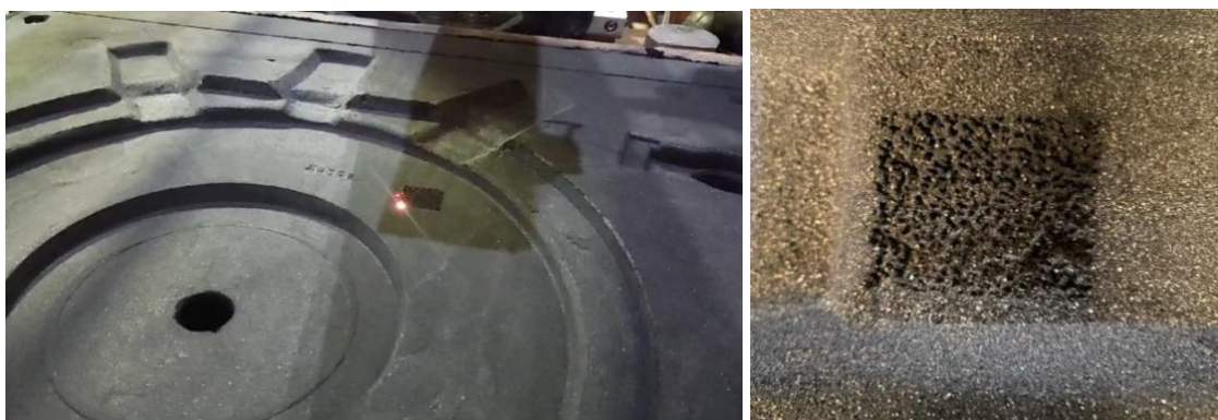
Figure 7 & 8: CDOT code second trial with 60W fiber laser with 110mm lens
