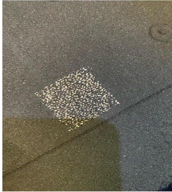
Figure 6: CDOT code first trial with 50W fiber laser with 300mm lens
