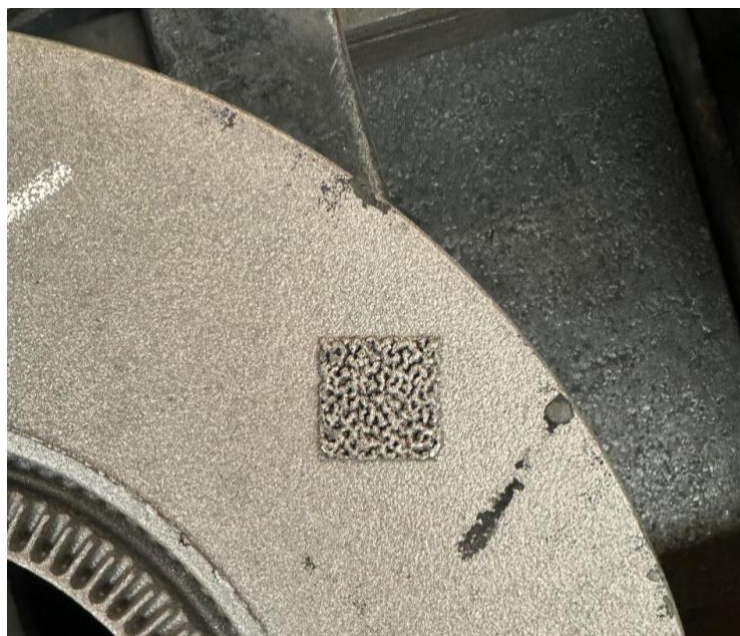
Figure 12: %100 readable CDOT code marked on sand mold, transferred to part during ore pouring
