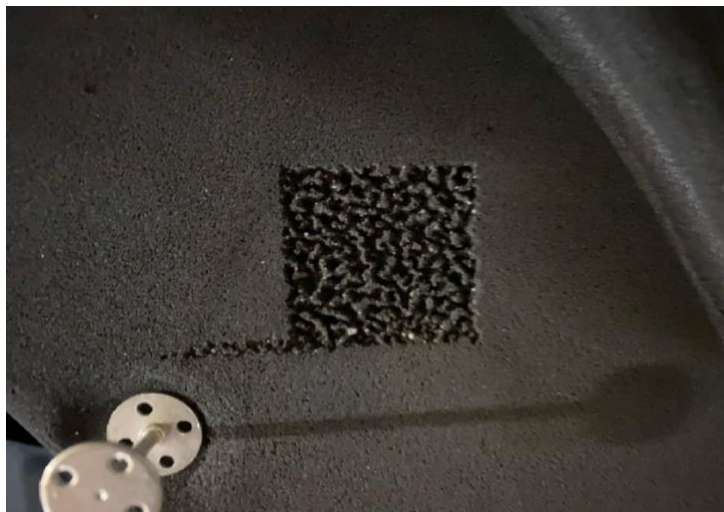
Figure 10: %100 Readable CDOT code engraved in the sand mold with 60W fiber laser and 110mm lens in the production
