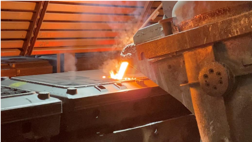
Figure 11: CDOT code transfer from sand mold to brake disc during pouring ore stage
